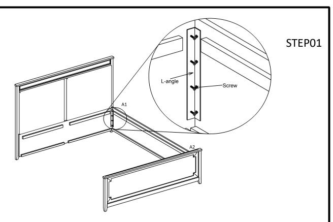
Fix the Part -A(Headboard),Part-B(Sideboard),Part-F(Footboard) using Langle with the help of Screw 16mm as shown in fig.
