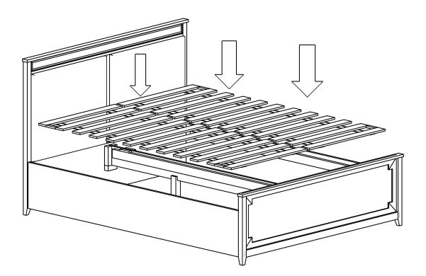
Now place Part-F(LVL Slates) into last assembled part as shown in fig.
