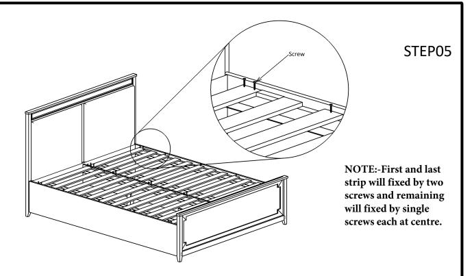
Now fix Lvl slates with last assemble part using screws of 25 mm at 1st ,3rd,6th,9th and 12th strip as shown in fig.
