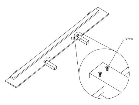
Now fix Part-C(Middle panel) and Part-D(Leg) with screw of 25 mm at position B1 and B2 as shown in fig.
