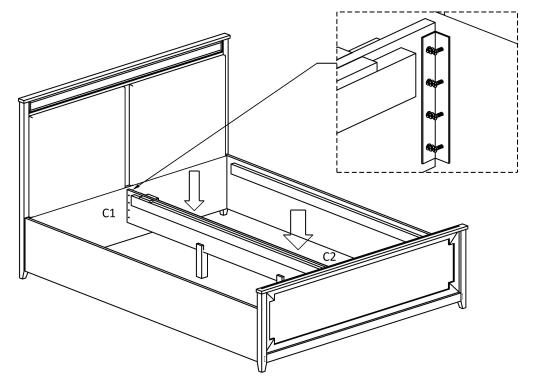
Now fix Part-C(Middle panel) with Part-A(Headboard) and Part-E(Footboard) using metal L-angle with screws 16 mm at position C1 and C2 respectively as shown in fig.
