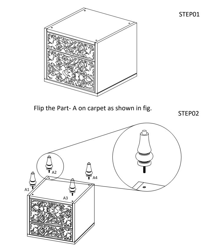
Fix Part-B(Leg) and Part -A(Cabinet) by rotating leg inside the stud in clockwise direction with D-nut at position A1,A2,A3 and A4 as shown in fig.
