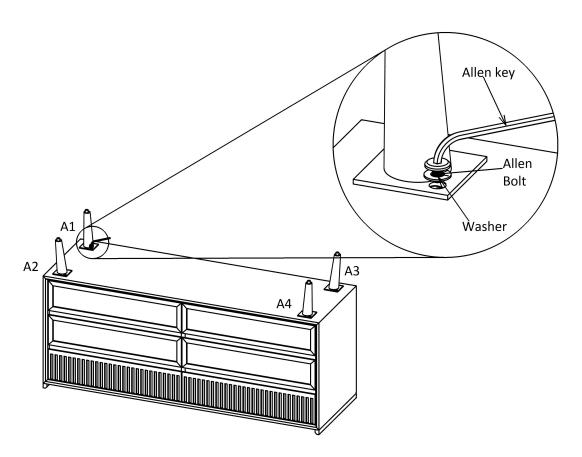
Fix the Part-B and Part -A with washer and allen bolt of M8x20 mm using Allen key at position A1,A2,A3 and A4 as shown in fig.
