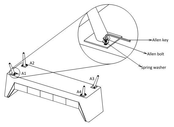
Fix the Part-B and Part -A with washer and allen bolt of M8x20 mm using allen key at position A1,A2,A3 and A4 as shown in fig.
