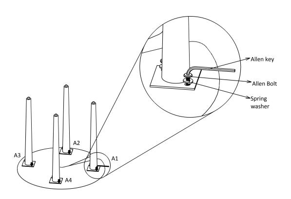
Fix the Part-B and Part -A with washer and allen bolt of M8x20 mm using Allen key at position A1,A2,A3 and A4 as shown in fig.
