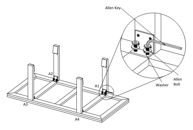
Fix the Part-B and Part -A with spring washer and allen bolt of M8x20 mm using allen key at position A1,A2,A3 and A4 as shown in fig.
