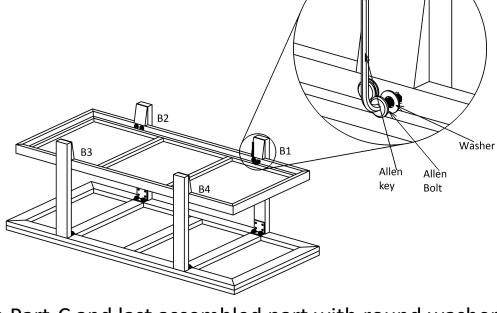
Fix the Part-C and last assembled part with round washer and allen bolt 35 mm using allen key at position B1,B2,B3,B4 respectively as shown in fig.
