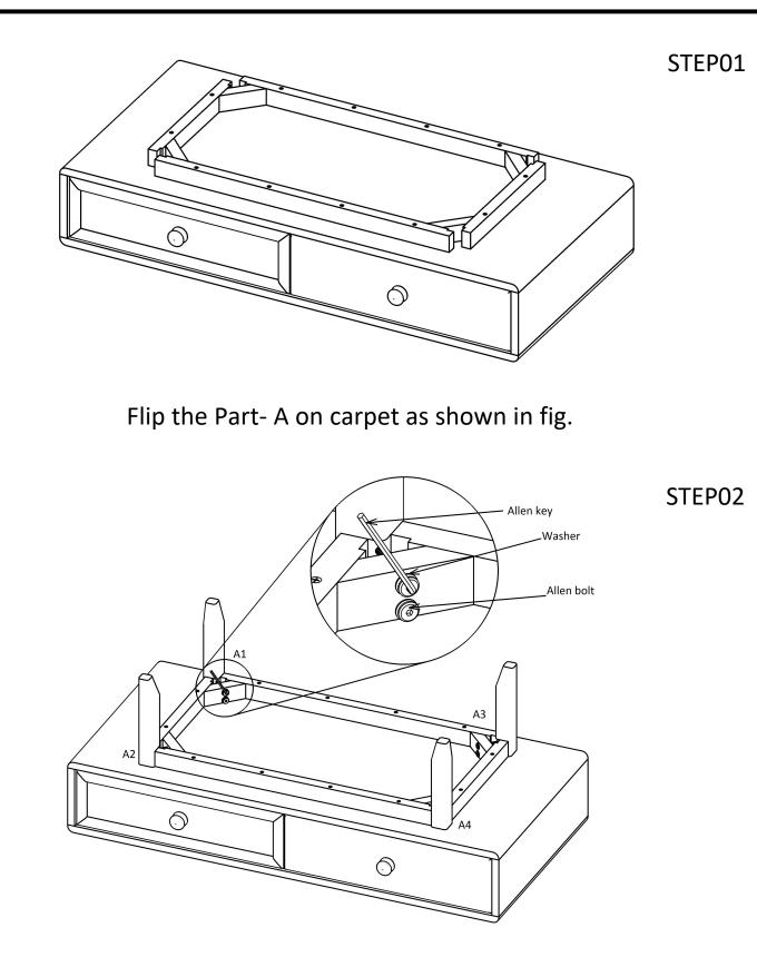
Fix the Part-B and Part -A with washer and allen bolt of M8x70mm using allen key at position A1,A2,A3 and A4 as shown in fig.
