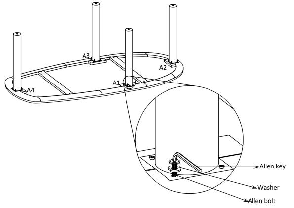
Fix the Part-B and Part -A with spring washer and allen bolt of M8x20 mm using allen key at position A1,A2,A3 and A4 as shown in fig.
