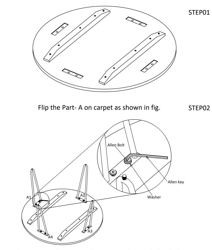
Fix the Part-B and Part -A with spring washer and allen bolt of M8x20 mm using allen key at position A1,A2,A3 and A4 as shown in fig.
