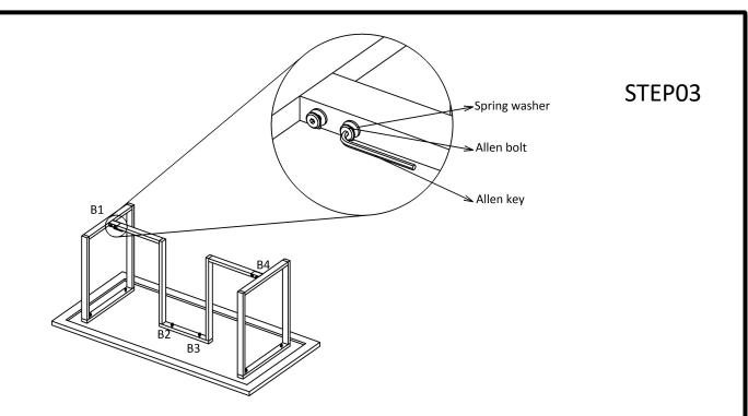
Fix the Part-C and last assembled part with spring washer and allen bolt 20 mm & 35 mm using allen key at position B1,B4 and B2,B3 respectively as shown in fig.
