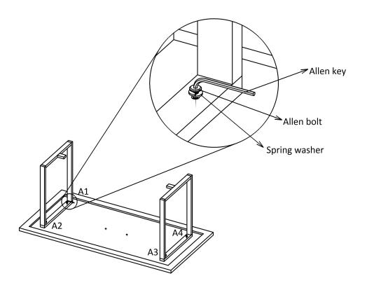
Fix the Part-B and Part -A with spring washer and allen bolt of M8x35 mm using allen key at position A1,A2,A3 and A4 as shown in fig.
