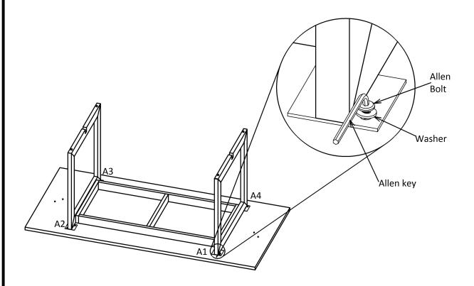
Fix the Part-B and Part -A with spring washer and allen bolt of M8x20 mm using allen key at position A1,A2,A3 and A4 as shown in fig.
