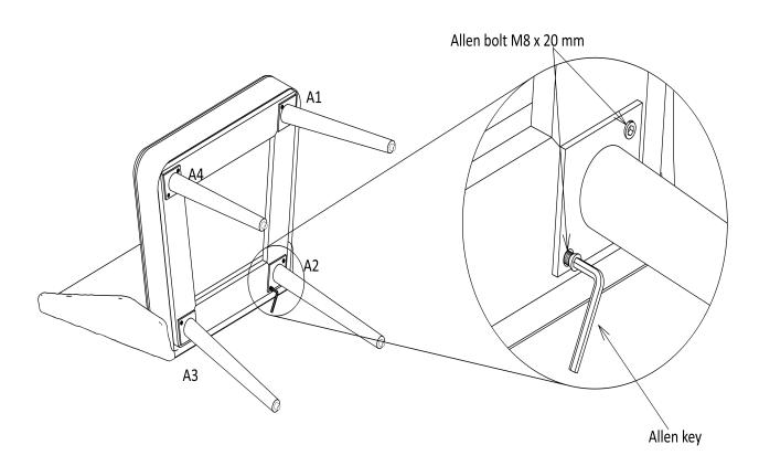
Fix the Part-A & Part-B with using Allen bolt M8x20 mm with help of Allen key at position A1,A2,A3&A4 as shown in Fig.
