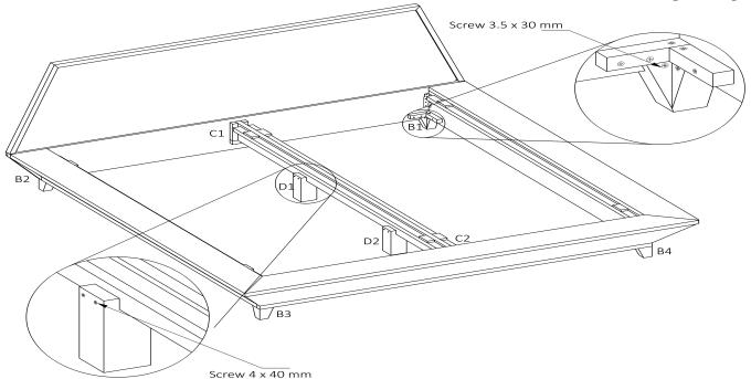
Fix the PART-C(leg) with last assembled part using screws of 30 mm with the help of screw driver at position B1,B2,B3 and B4.Now place part D at position C1 and C2 respectively as shown in fig. and fix the PART-E(center leg) using screws of 40 mm.
