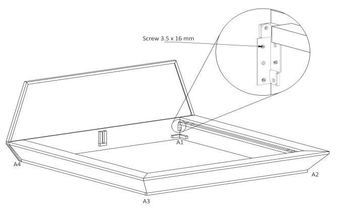
Fix the PART-A, PART-B and PART- E with bed clamp using screw of 16 mm at position A1,A2,A3 & A4 as shown in Fig.
