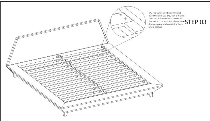
Place the Part-F(strips panel) on last assembled part as shown in Fig.
