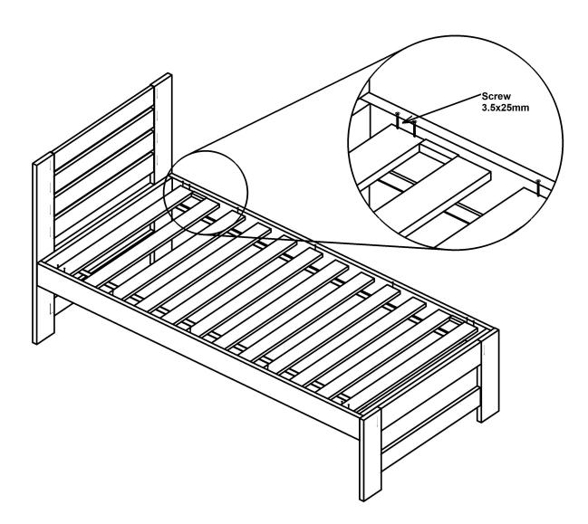
Note:-1st and last slates have double screw and remaining slates have single screw
