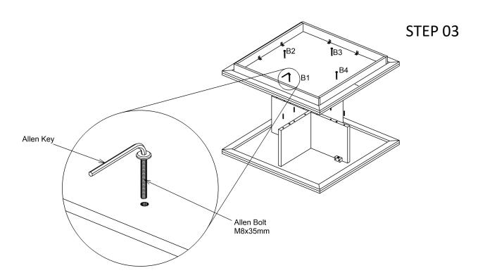
Now place PART-D(Bottom) with last assemble part and fix with dowel & allen bolt M8X35mm using allen key at position B1,B2,B3 &B4 as shown In Fig.
