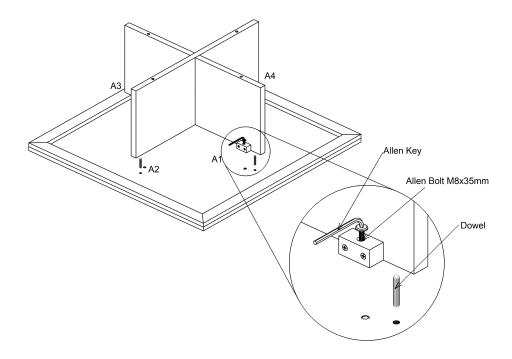
Flip the PART-A(Top) and last assembled part on carpet and fix with dowel & allen bolt of M8x35mm using allen key at position A1,A2,A3 and A4 as shown in Fig.
