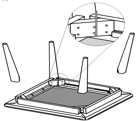
Fix Part B (Leg) with Allen bolt using Allen key as shown in Fig.
