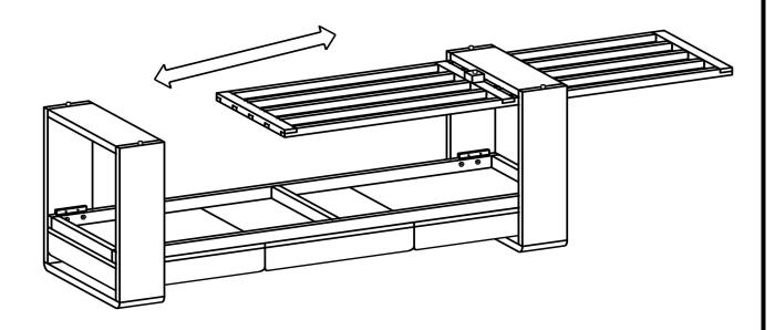
Insert Part C in last Assemble part as shown in fig.
