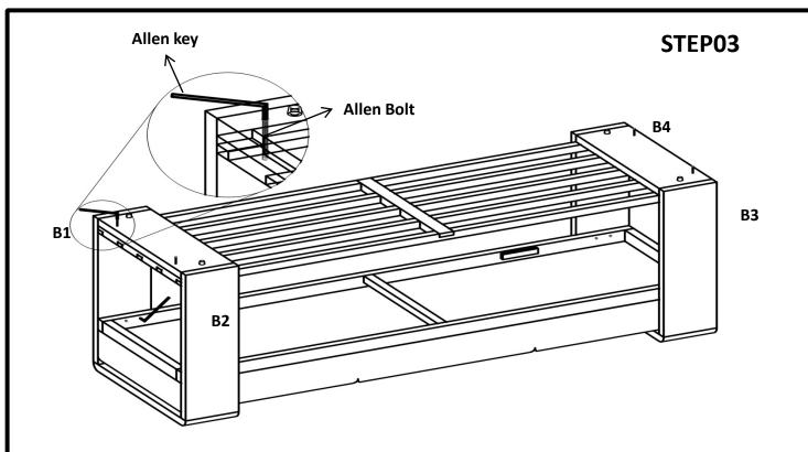
Fix part c using Allen bolt at position B1,B2,B3 &B4 with the help of allen key as shown in fig.
