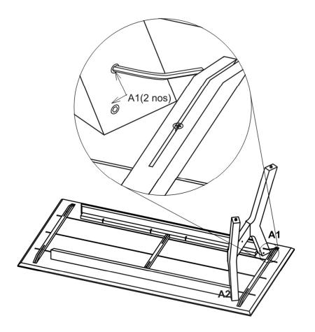
Fix PART-A and PART-C(one side) with Allen bolt using Allen key at defined Position A1 and A2 as shown in Fig.
