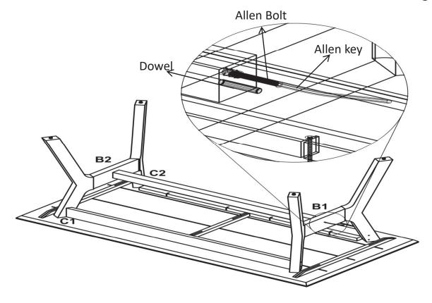
Fix PART-B with last assemble Part with allen Bolt Using Allen key At position B1,B2. Also PART- C(Other side) at C1 &C2 similar to STEP 02 as shown in Fig.
