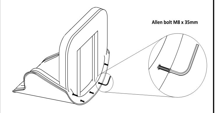
Fix the Part-A & Part-B with using Allen bolt -35mm with help of Allen key at Five position as shown in Fig.
