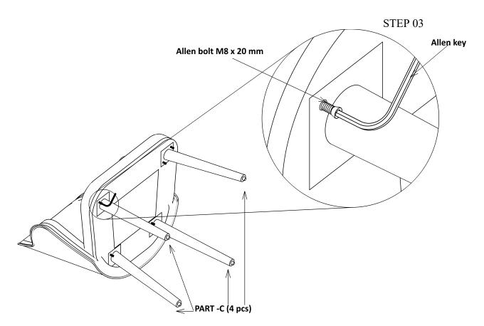
Fix the Part-C & last assembled part with using Allen bolt - 12mm with help of Allen key as shown in Fig.
