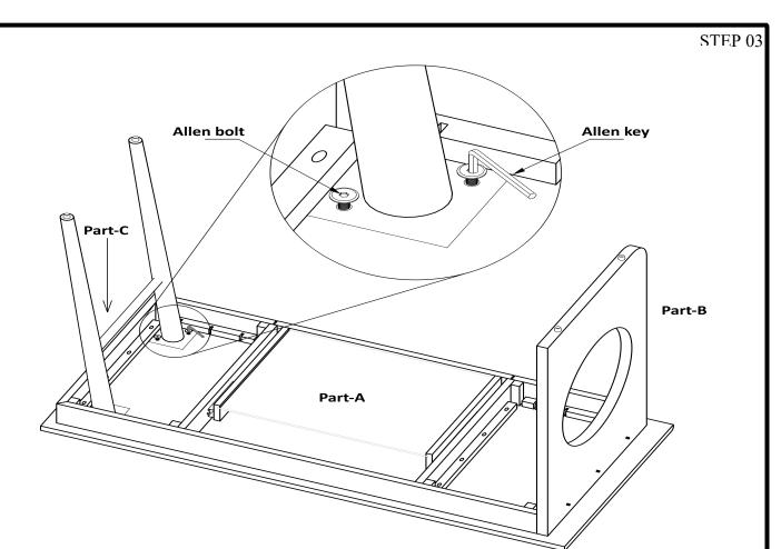
Fix the Part-C & last assembled part by Allen bolt- 12 mm with help of Allen key as shown in Fig.
