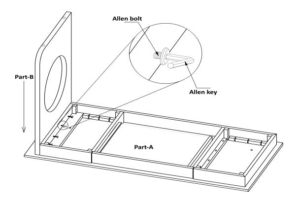
Fix the Part-A & Part-B by Allen bolt-35 mm with help of Allen key as shown in Fig.
