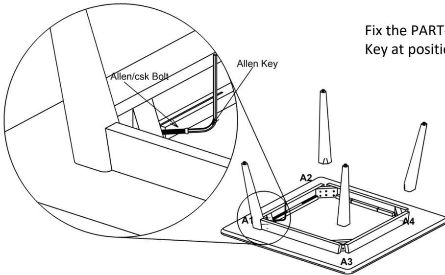
Fix the PART-B (leg) with Allen Bolt using Allen Key at position A1,A2,A3 & A4 as shown in Fig.
