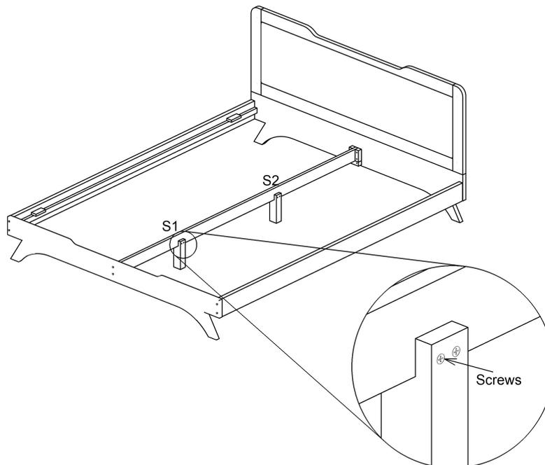
Fix the Part-D(Leg) with screw of 25 mm at position S1&S2 as shown in Fig.
