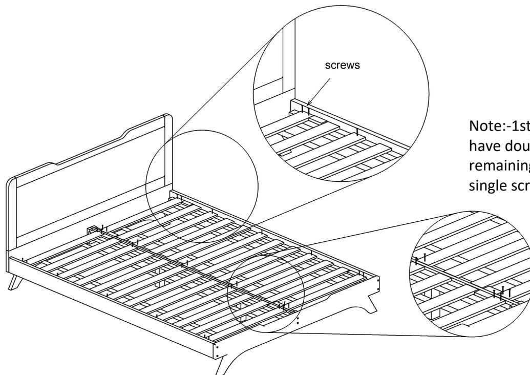
Note:-1st and last slates have double screw and remaining slates have single screw
