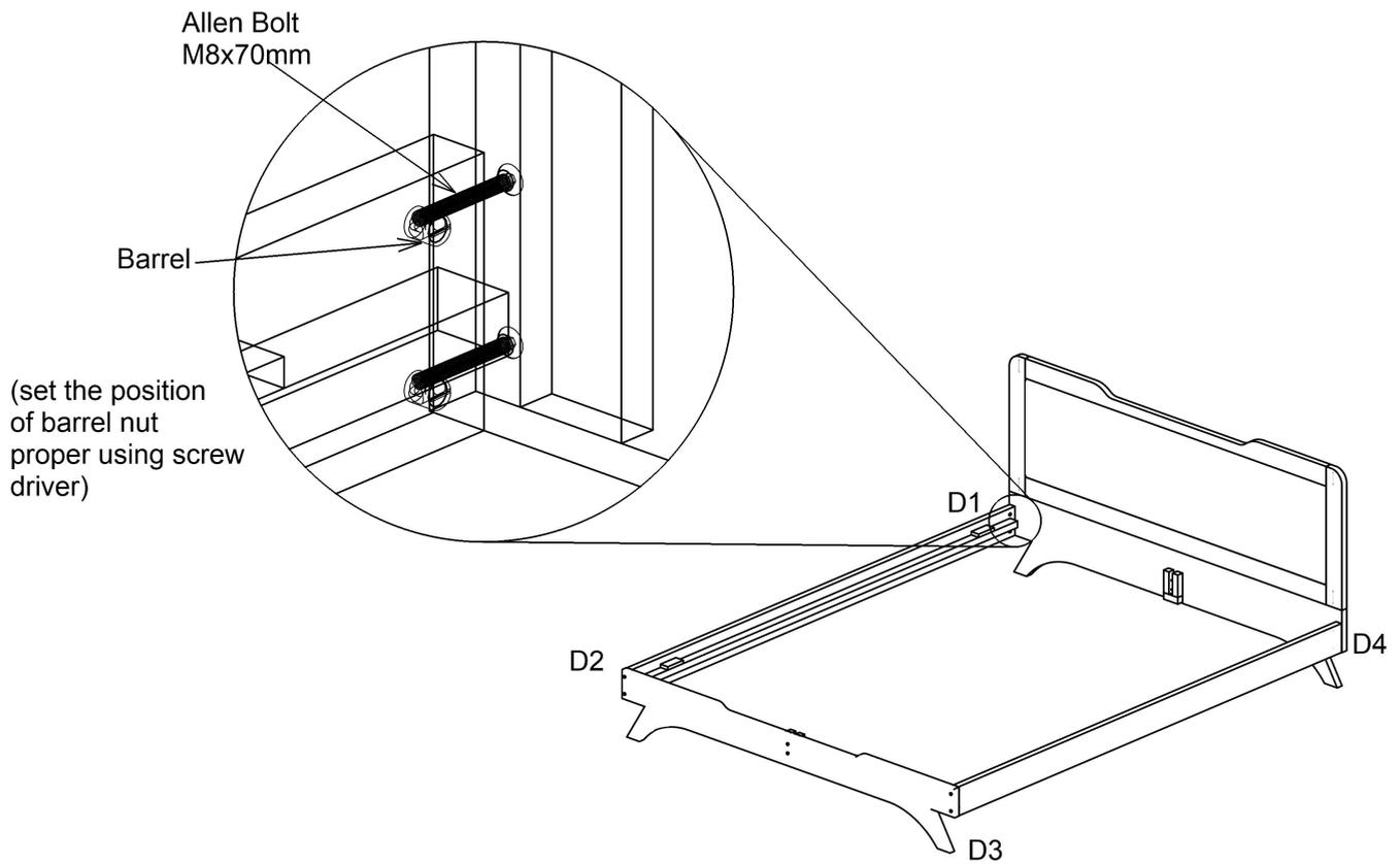
Fix the Part -A(Headboard),Part-B(Sides)&Part-E(FootBoard) with barrel nut and allen bolt with the help of allen key at defined position D1,D2,D3,& D4 as shown in fig.
