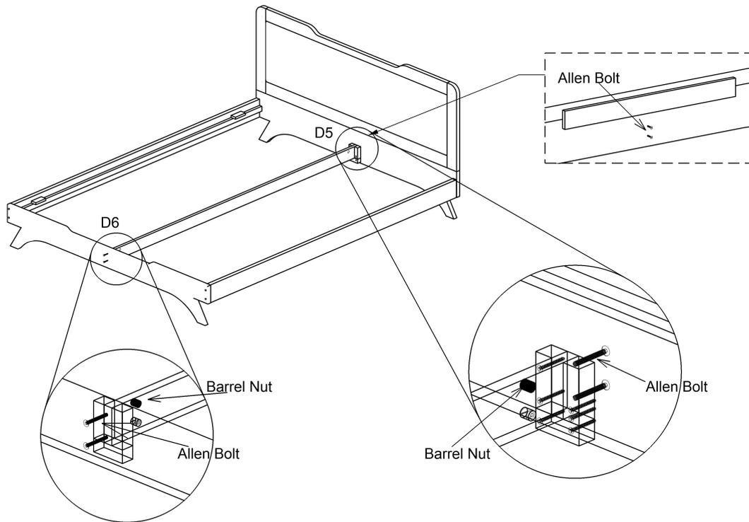
Fix the Part-C (middle part) with barrel nut and allen bolt at position D5 & D6 similar as STEP01 as shown in fig.
