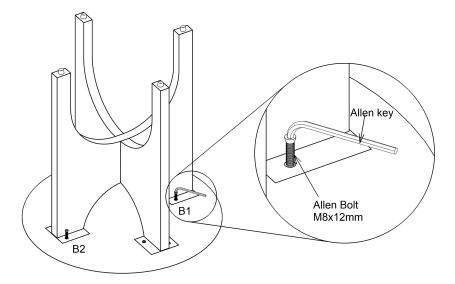
Fix the Part-C with last assembled part with allen bolt of M8x12mm using allen Key as shown in fig.
