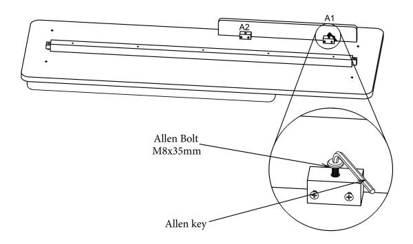
Fix the Part-A & Part-B with using Allen bolt with help of Allen key at position A1&xA2 as shown in Fig.
