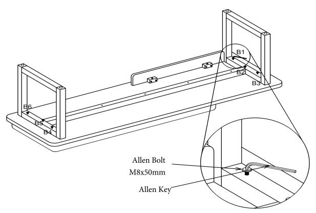
Fix the Part-A & last assembled part with using Allen bolt with help of Allen key at position B1,B2,B3,B4,B5&B6 as shown in Fig.
