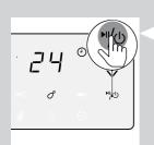
4 Press the On/Off button to start the cooking process.
