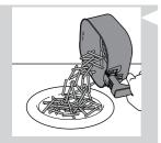
12 Empty the basket contents into a bowl or onto a plate. Always remove the basket from the pan to empty contents as hot oil may be in the bottom of the pan.
