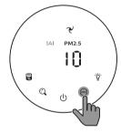
Gentle mode ( で): The air purifier operates at a low speed.
