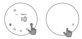
You can touch the light on/off button  $\overset{\circ}{\nabla}$  manually to turn off all lights and the control panel. Touch any button to wake up all lights.
