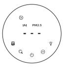
The "---" displays on the screen during warming up. Then the air purifier shows the PM2.5/IAI level after measuring the air quality.
