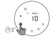
Touch and hold the filter status check/reset button for 3 seconds to reset the filter cleaning time.
