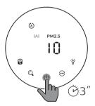
Touch and hold the button for 3 seconds to switch off the air purifier.
