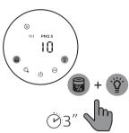
Within 15 seconds after power on, touch and hold and button for 3 seconds to reset the filter lifetime counter.
