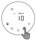
Auto mode ( ((a)): The air purifier automatically adjust the fan speed in accordance with the ambient air quality.
