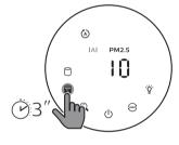
3 Touch and hold the filter status check/ reset button a for 3 seconds to reset the filter cleaning time.
