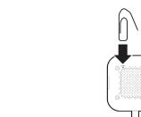
**Step 2:** Use a pin to press the Reset button for 5 seconds until the camera starts to beep.
