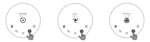
Auto mode ( ((a)): In Auto mode, the dual-sensor senses the air quality in real-time and the appliance automatically adjusts the fan speed in accordance with the ambient air quality.
