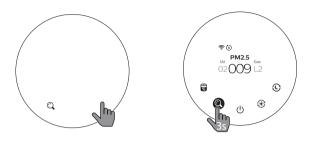
With the light sensor, the control panel can automatically turn on, turn off or dim according to the ambient light. The control panel will be off or dim when the ambient light is dark. You can touch any button to wake up all lights. Then, if no further operation, all lights will be off or dim again to match with the ambient light. You can touch and hold the C button for 3 seconds manually to turn off all lights and the control panel. Touch any button to wake up all lights.
