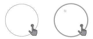
**Normal Sleep mode:** In normal Sleep mode, the air purifier operates quietly at a low speed. After 3 seconds, the **O** button dims, all lights and buttons are off.
